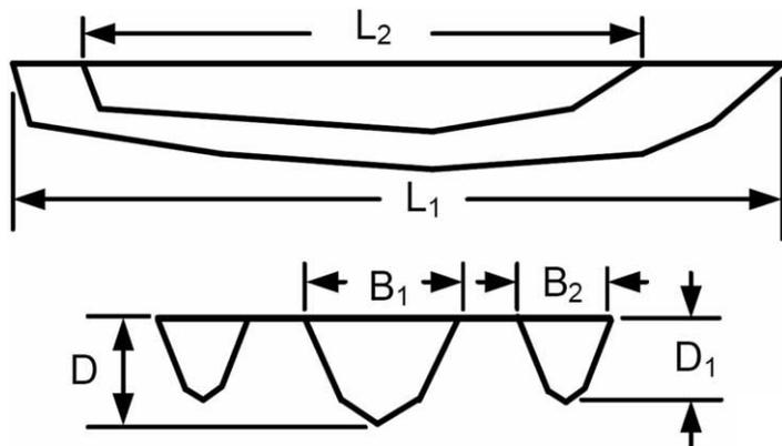
12.5 ft. Beam x 7.25 ft. Depth of Hull/100 = 19.1 tons
