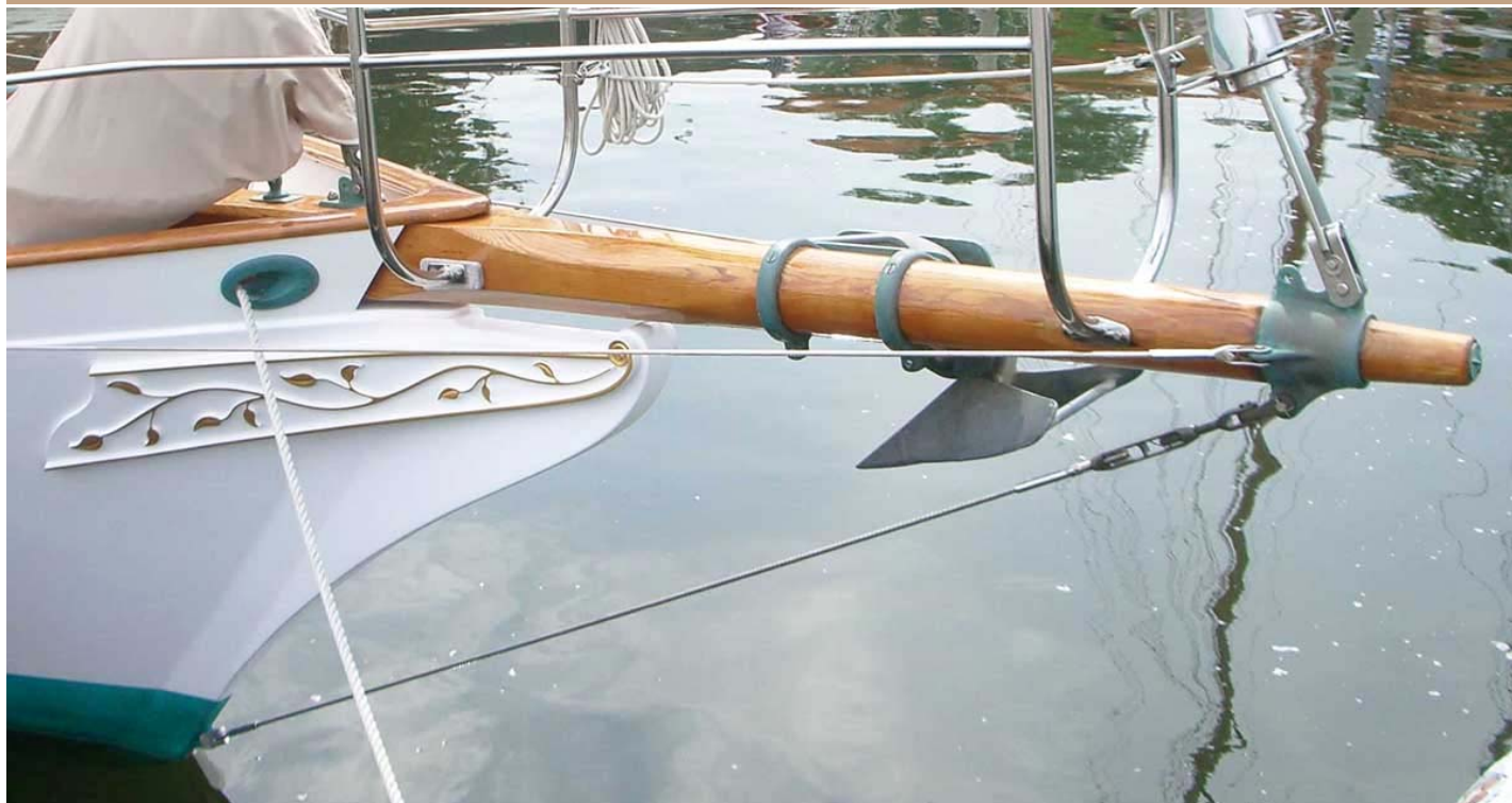
Bronze Kranz Iron, Anchor Roller, and Hawse Holes, with Stainless Steel Stanchions and Rod Rigging
