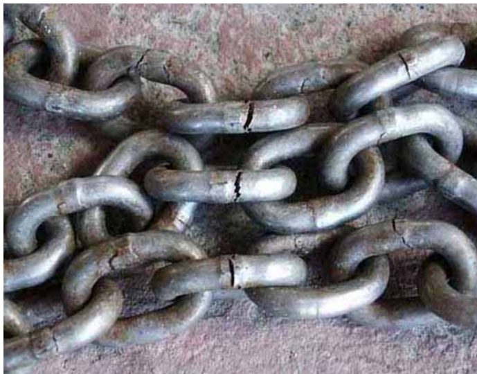
Stainless Anchor Chain Failure At Welds
