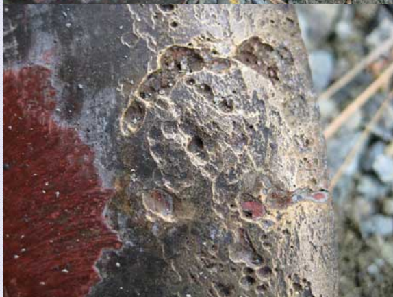
Severely Corroded Bronze Propeller
