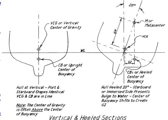
the same spot at small angles of heel (under 10 degrees) and then it gradually begins to shift location. Regardless, to determine stability you have to find the metacenter and the vertical center of gravity, VCG.
